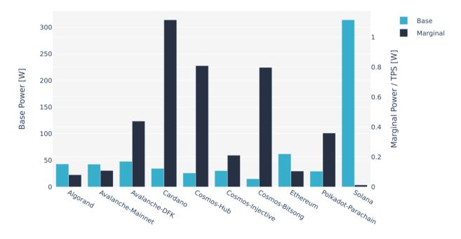
Figure 3: Base power demand and marginal power demand per TPS for a best guess single node of the respective network in watts.
