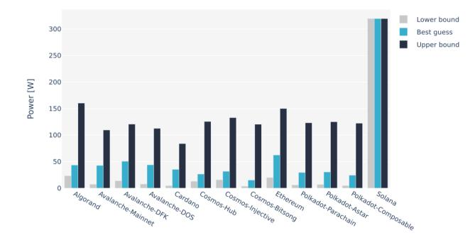
Figure 2: Overview of lower bound, upper bound and best guess power demand estimates for a single node of the respective network in watts.
